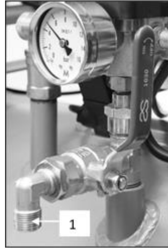
Fig. 8: Connecting to the compressed air outlet
