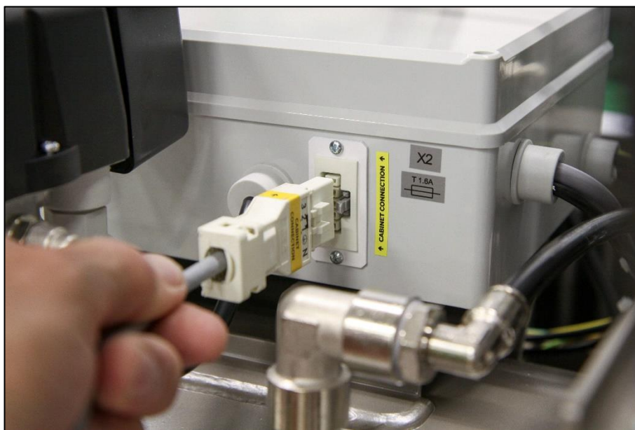
Fig. 13: Connect the cabinet to the compressor
