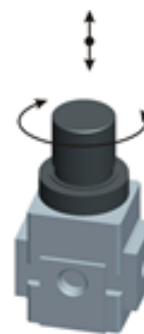
Fig. 15: Setting outlet air pressure
